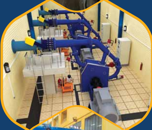
Ready to Execute Design with Pelton Turbines (up to 6 MW)
