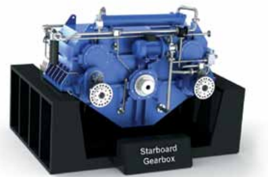
▶ Design of 10 megawatts of CODAD Gearbox
